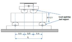
Fig 3.2 Diagrammatic view of flexure test of concrete by third-point loading Method
